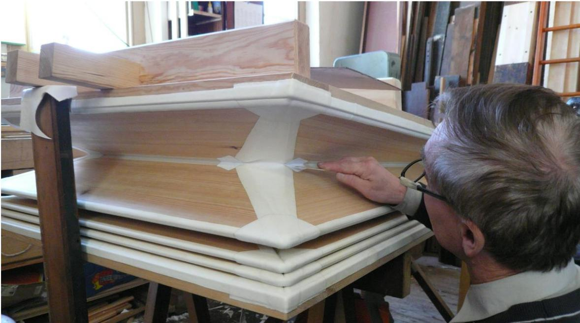
A wedge shaped cut-out in one building-frame upright confirmed that the original bellows would have been placed with their hinges towards the front of the organ. This arrangement meant that hand-pumping could be done best by pulling them up with ropes and pulleys. Levers over the top as shown in some illustrations of similar bellows, would be pointing the wrong direction.
