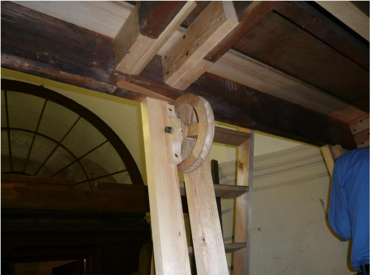
By employing a second pulley at the bellows attachment, the force required to raise the bellows is reasonable. Keeping the organ supplied with wind manually is not too demanding. The size of the non-return valves is such that at least two bellows have to be supplying at the same time, in order to be able to supply enough wind for the full organ.
