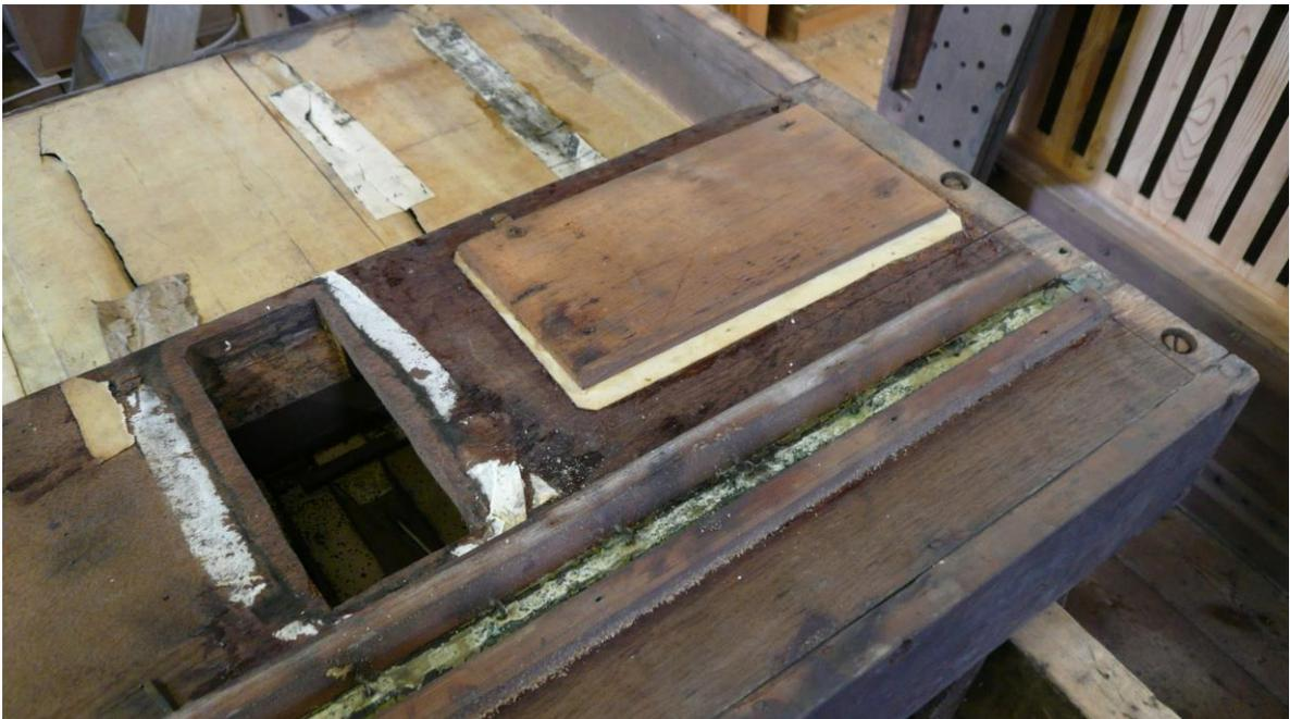
The Great has two trunks (+2600mm long) with an inside cross section of approx. 222mm x 98mm. The Choir has two trunks that branch off about 755mm from the top of the Great trunks with a cross section of 190 x 91mm.
