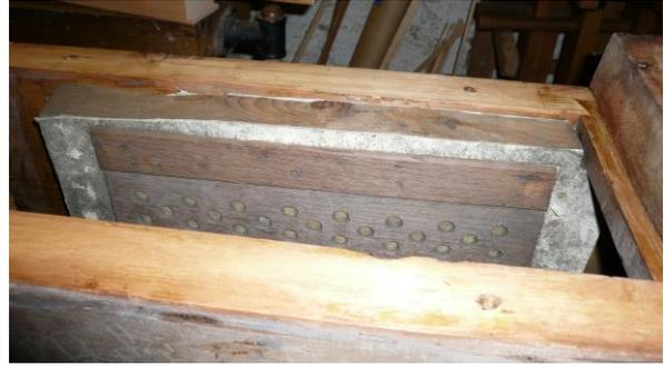
Installed wind system with service hatch removed showing the restored non-return valve
