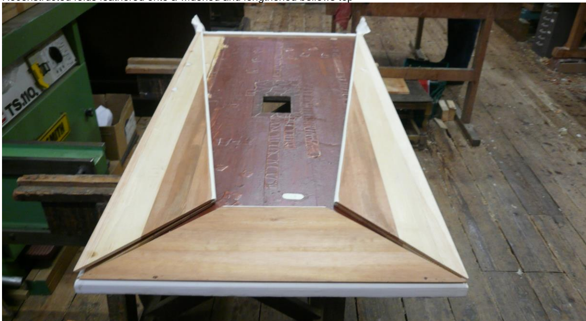
Reconstructed folds leathered onto a widened and lengthened bellows top
