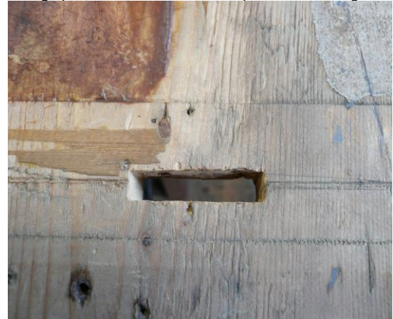
Remains of the leather strap hinges wedged into the valve board. A hinge pocket cleaned out and a splinter of the hinge-slat
