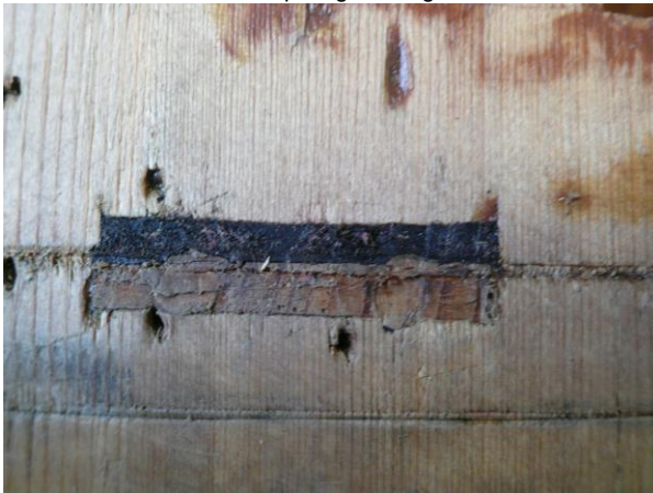
Remains of the leather strap hinges wedged into the valve board. A hinge pocket cleaned out and a splinter of the hinge-slat
