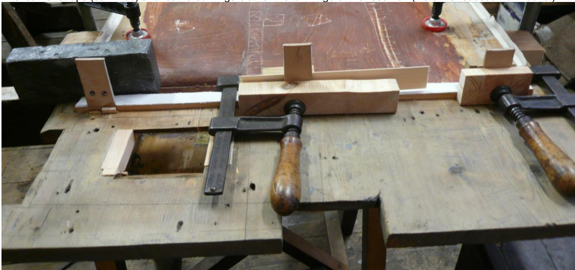
The leather straps (cow hide) and leatherned hinge-slat for the tail hinge of the reservoir (Note the reduced trunk outlet)
